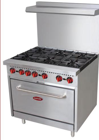
The Entrée Sauté Commercial Gas Range has powerful Planck 30,000 BTU cast iron burners. Each burner has an individual pilot light - heavy duty 12" x 12" removable cast iron grate and individual instant light control knob. It is constructed with a stainless steel front, 24.75" high backriser and shelf, 6" adjustable stainless steel legs or casters and a 34" NPT gas connection.
